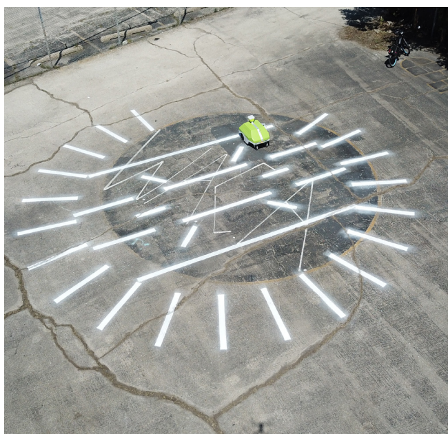
Figure 3. View of painting robot installing the pattern. Image by authors.
